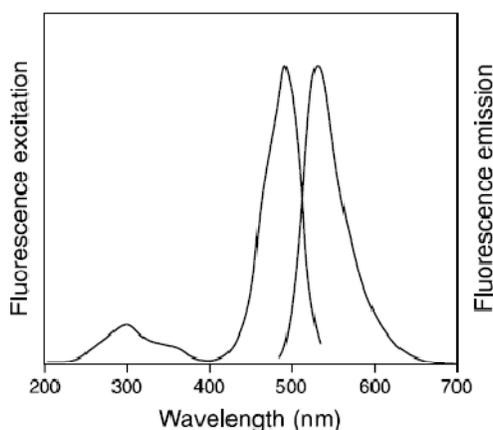
Figure 1. Spectra of SYBR Gold nucleic acid gel stain bounding with double-stranded DNA.
