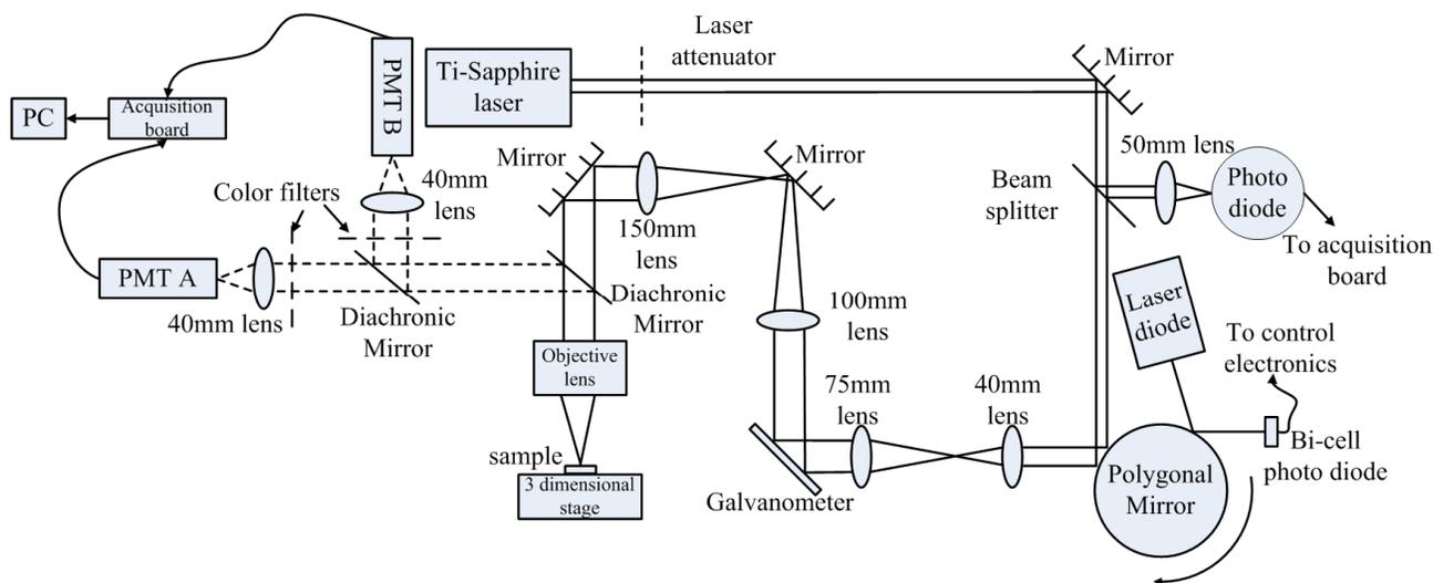
Figure2. Schematic drawing of two-photon laser scanning fluorescence microscopy. PMT: photo multiplier tube. PC: personal computer.
